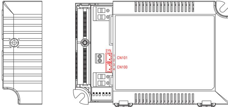
SYN+ or DC 0-10V Dimming Connector(CN101/CN100): JST B2B-XH or equivalent
