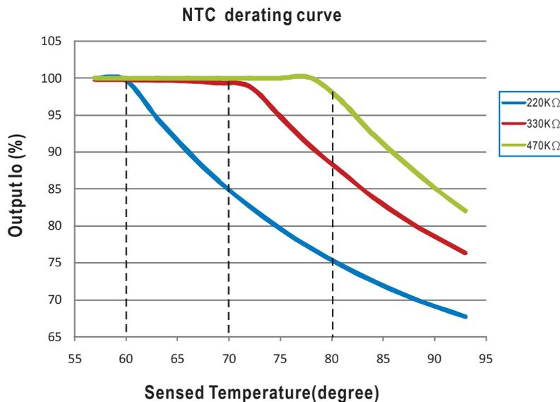
LCM-40EO have the built-in temperature compensation function ( $T \uparrow, I_o \downarrow$ ). By connecting a temperature sensor (NTC resistor) between the NTC +/- terminal of LCM-40EO and the detecting point on the lighting system or the surrounding environment, output current of LCM-40EO could be correspondingly changed to ensure the long life of LED.
