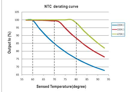
LCM-60EO have the built-in temperature compensation function (T \( \cdot, lo \( \preceq \)). By connecting a temperature sensor (NTC resistor) between the NTC +/terminal of LCM-60EO and the detecting point on the lighting system or the surrounding environment, output current of LCM-40EO could be correspondingly changed to ensure the long life of LED.
